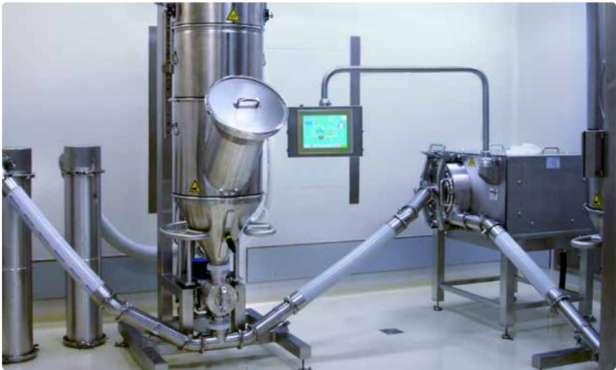
REKORD 315 GMP fine grinding system for cell culture feed
