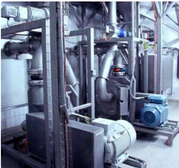
REKORD 630 GMP fine grinding system for lactose
